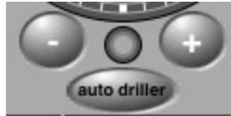
It is necessary to tap on buttons - / + to maintain the **WOB** (weight on bit).
