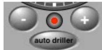
The **WOB** (weight on bit) is constant. It changes automatically to Off if to tap on the buttons - / +
