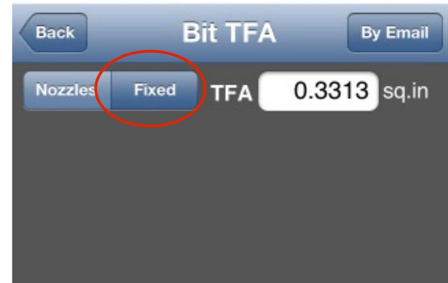
$$\text{Bit Loss} = \frac{\text{MW} \times \text{Flow}^2}{12032 \times \text{Coeff}^2 \times \text{TFA}^2}$$
